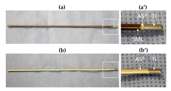
**Figure 1.** (a) Test item: SML-coated  $AS^{\mathbb{R}}$ /titanium K-wire, (a') shows the two coatings in magnification. SML = bronze,  $AS^{\mathbb{R}}$  = golden. (b) Blank item:  $AS^{\mathbb{R}}$ -coated titanium K-wire, (b') shows the  $AS^{\mathbb{R}}$  coating in magnification. The silver color at the blunt end of each K-wire shows the uncoated titanium surface.
