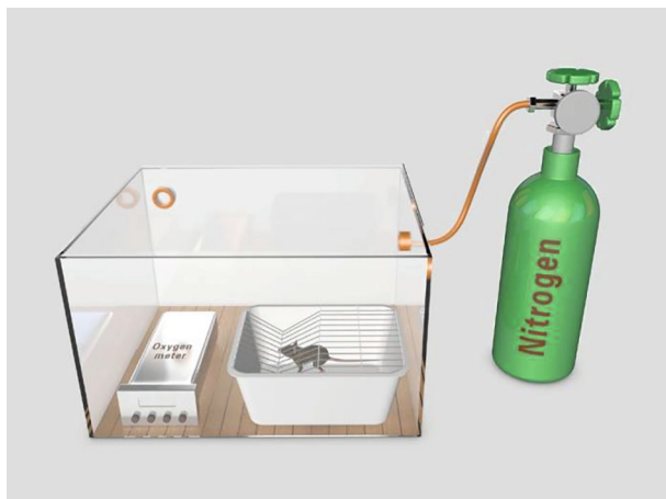
FIGURE 1: The hypoxia mechanism: It was a 60 × 80 cm plastic box. Nitrogen was pumped for adjusting the concentration of oxygen (10–12%) in the box. An oxygen meter was put for monitoring.
