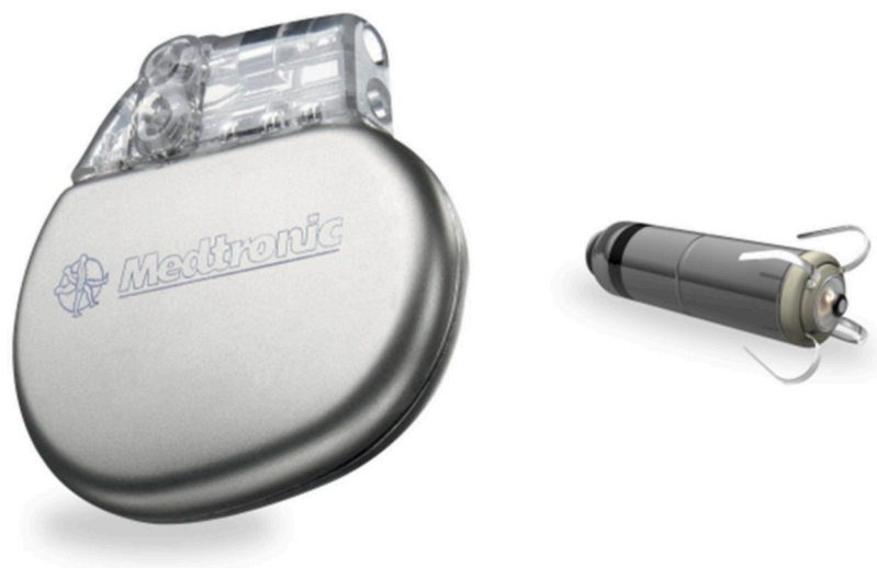
Figure 1. A typical dual-chamber pacemaker ( left ) and the Micra ( right ). Reproduced with permission from reference [26] and Medtronic, Inc.
