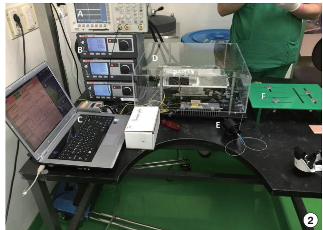
Fig. 1. Schematic view of the 3-stage YDF MOPA system: (1) schematic plot, (2) pictures of real products. (A) Oscilloscope (TDS3032B, Tektronix, Beaverton, OR, USA). (B) Pump laser diodes (LDC 4020, Thorlabs, Newton, NJ, USA). (C) Laptop seed laser driver (SLDD401P, NOTICE, Anyang, Korea). (D) Three-stage YDF MOPA system (made in-house). (E) Focuser tip (focal length, 47 mm; spot size, 5 μm). YDF MOPA, ytterbium-doped fiber master-oscillator power amplifier; TFB, tapered fiber bundle; LD, laser diode.
