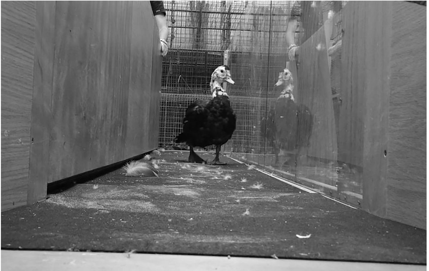
Fig 1. Pressure sensitive walkway. Muscovy duck ( Cairina moschata domestica ) on pressure sensitive walkway (PSW) within a custom-designed chute composed of wooden and acrylic panels.
