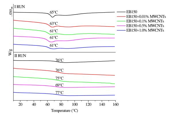
**Figure 8.** DSC traces (1st and 2nd heating up) for UV-LED cured EB150 and its composites with different MWCNTs loadings.
