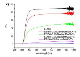
**Figure 11.** UV-Vis spectra of films containing (**a**) MWCNTs, (**b**) BC and (**c**) BC/MWCNTs in concentrations ranging from 0.01 to 1.00 wt%.
