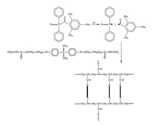
**Figure 1.** Scheme of UV-LED curing of EB150. The system undergoes a radical polymerization promoted by the generation of primary radicals derived from the photolysis of the photoinitiator as a consequence of the exposure to the UV-LED radiation.
