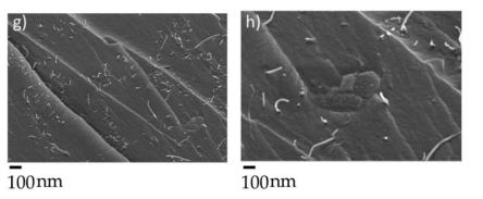
**Figure 5.** FESEM captures of UV-LED cured films (filler loading: 1 wt%): unfilled EB150 (**a**,**b**); EB150 + MWCNTs (**c**,**d**); EB150 + biochar (**e**,**f**) and EB150 + biochar/MWCNTs (**g**,**h**). All the filled UV-LED cured films show a good dispersion of the two carbonaceous fillers.
