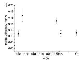
**Figure 10.** Thermal conductivity of UV-LED cured EB150 and its composite films as a function of filler loading: (**a**) with MWCNTs, (**b**) with biochar and (**c**) with biochar/MWCNTs. Different trends can be observed, according to the filler type and loading.
