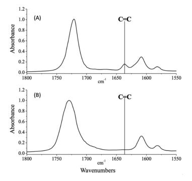
**Figure 2.** FTIR-ATR spectra of EB150 containing 0.50 wt% of biochar, before (**A**) and after (**B**) exposure to the UV-LED radiation. The disappearance of the band of the acrylic double bonds, located at about  $1635 \text{ cm}^{-1}$ , is a clear indication of the completeness of the UV-LED curing process.
