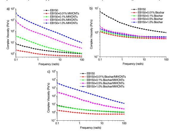
**Figure 6.** Complex viscosity vs. frequency curves for unfilled EB150 and EB150 + MWCNTs (**a**), EB150 + biochar (**b**) and EB150 + biochar/MWCNTs (**c**) at different loadings ranging from 0.01 to 1.00 wt%.
