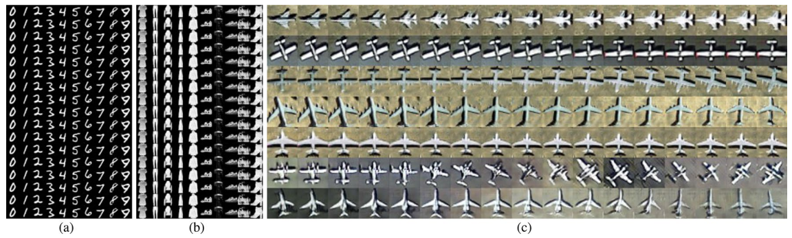
Figure 8. The potential space representation of 17 points between two random vectors z_i indicates that the interpolation space has learned smooth and meaningful semantic information transitions based on the same pair of latent variables, allowing nice inter-class interpolation.
