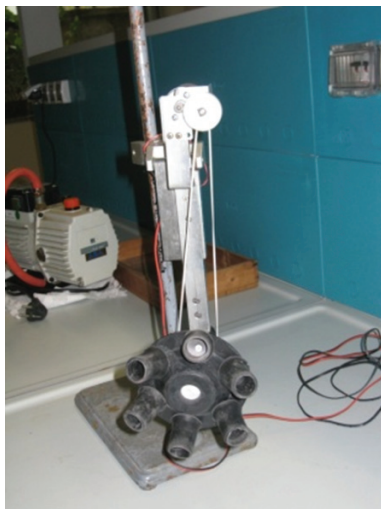
FIGURE 1: In vitro release apparatus: instrument at rotational motion in order to simulate mechanical stress in a vaginal environmental.
