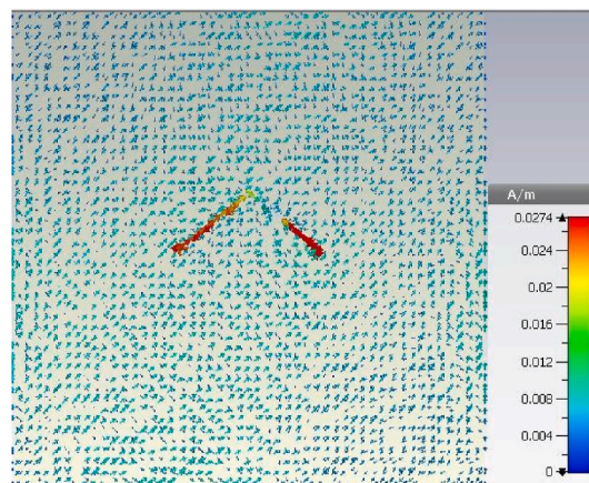
Fig. 5. Surface current distribution of the slot resonating at 28.87 GHz.
