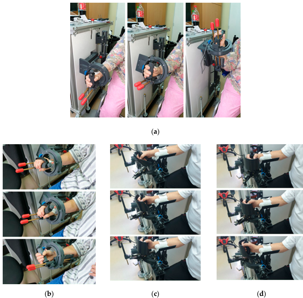
Figure 11. Snapshots from the experimental tests using ParReEx ((a) ParReEx-elbow flexion/extension, (b) ParReEx-elbow pronation/supination, (c) ParReEx-wrist adduction/abduction, (d) ParReEx-wrist flexion /extension).
