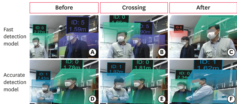
Fig. 2. Evidence of object tracking by the accurate detection model. Before indicates ‘before crossing’ and after indicates ‘after crossing.’ ‘Crossing’ indicates the moment just before the actual crossing. (A) had ID of 0 (green) and 5 (blue). (C) had ID of 0 (green) and 8 (red). The ID has changed after crossing for the fast detection model. However, for the accurate detection model, the ID remained the same after crossing. (D) had ID of 0 (green) and 1 (blue). Similarly, (F) had ID of 0 (green) and 1 (blue).
