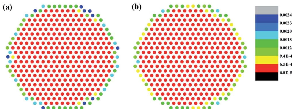
Fig. 4 Spatial distribution of localized phonon modes in diamond SLNWs at the interface atom layer (a), and at the non-interface atom layer (b). Positions of the circles denote the atom locations on the XY plane, and spatial distribution of localized phonon modes is depicted according to the colour.
