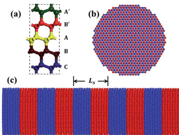
Fig. 1 (a) The structure of diamond SLNW. (b) The cross section of diamond SLNW. (c) The vertical axis plane of diamond SLNW.
