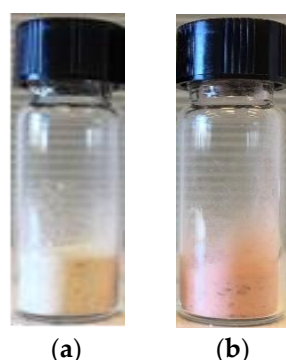
Figure 1. Photographs of the products after cross-linking reaction between thiophene grafted (a) and imidazole grafted; (b) products with BM.
