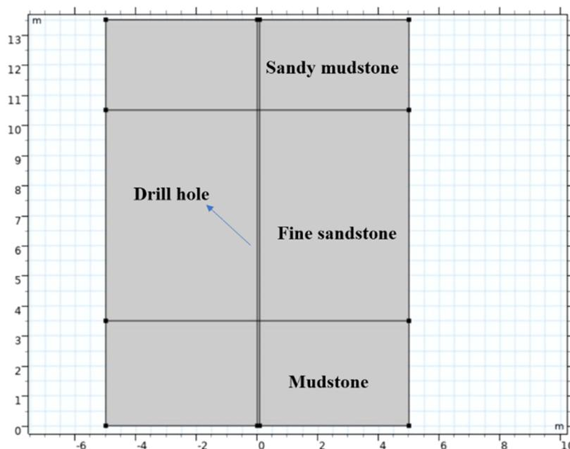
Figure 2. Model of numerical simulation.
