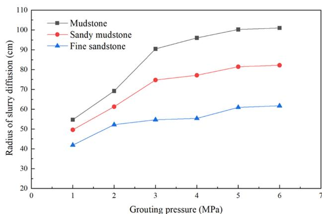
Figure 8. Grout diffusion radius under different grouting pressures.
