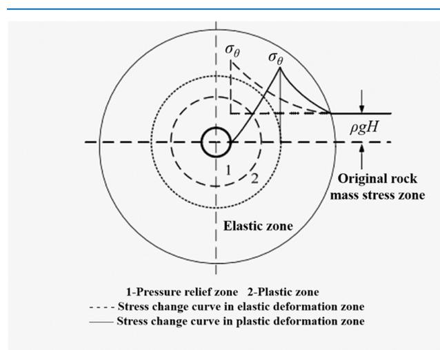
**Figure 1.** Stress distribution around the borehole.
