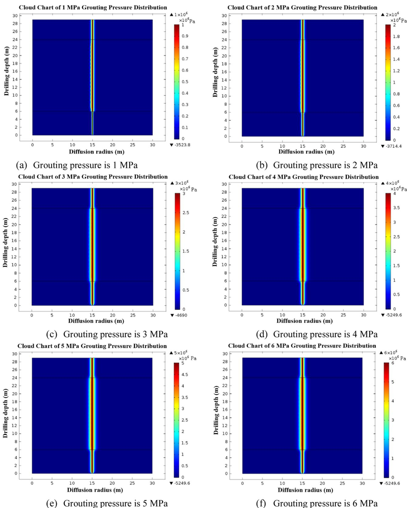
Figure 6. Slurry pressure distribution under different grouting pressures.
