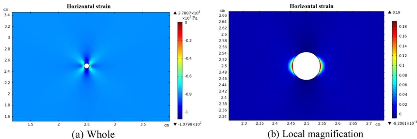
**Figure 3.** Horizontal stress changes after the formation of a borehole.
