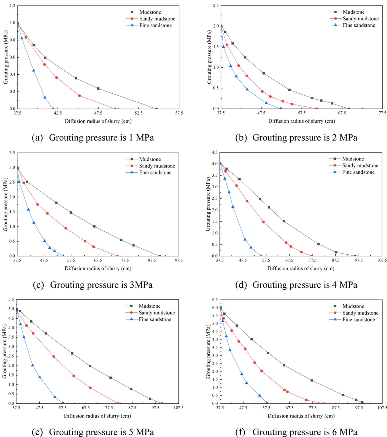
Figure 7. Attenuation diagram of grouting pressure with diffusion radius.
