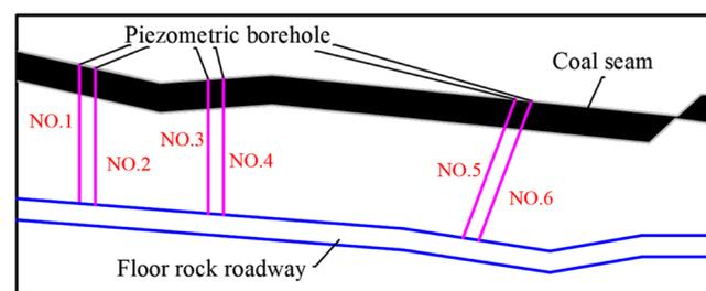
Figure 9. Specific location of pressure measuring borehole.
