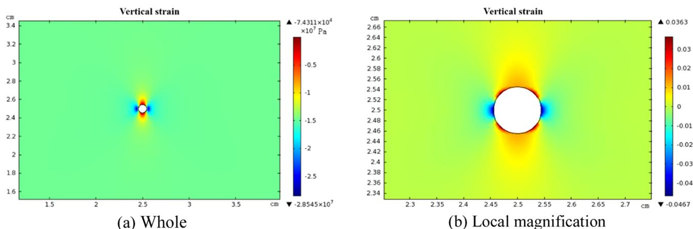
Figure 4. Vertical stress map after the formation of a borehole.
