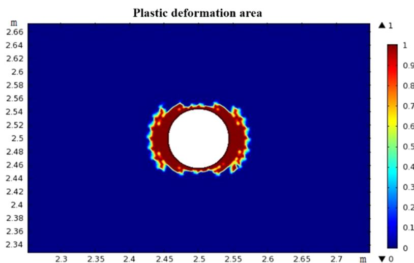
Figure 5. Plastic damage area around the borehole.
