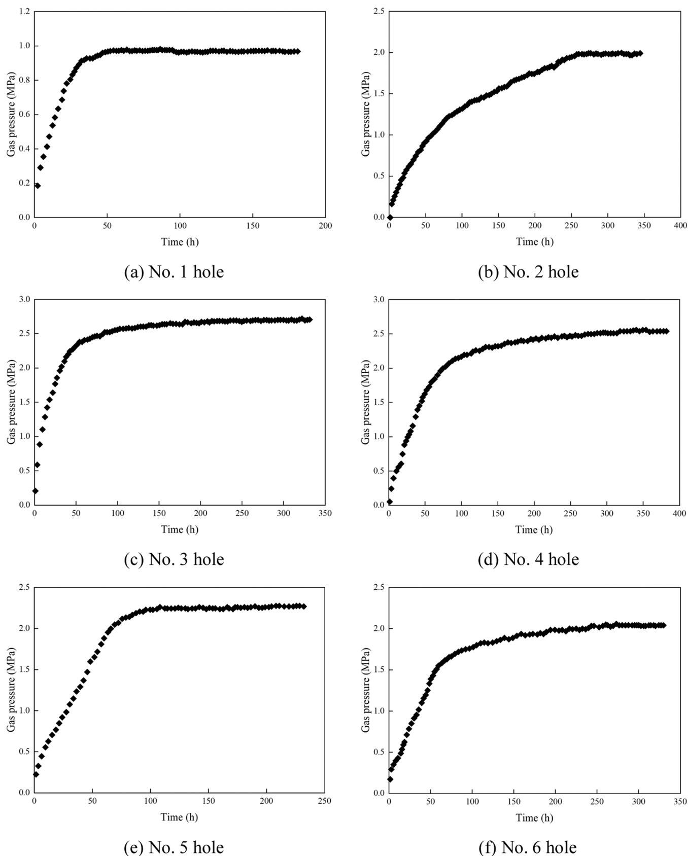
Figure 10. Gas pressure recovery curve of boreholes.
