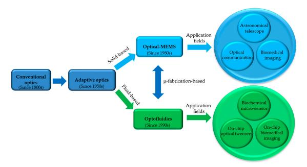
**Figure 1.** The evolvement of optofluidics from conventional optics with its applications in the fields of biochemistry, biomedical engineering, analytical chemistry, etc.
