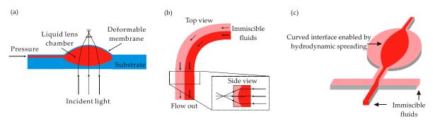
**Figure 4.** Illustration of optofluidics lenses: (**a**) out-of-plane lens tuned by applying pressure on a deformable membrane; (**b**) in-plane lens enabled by Dean flow; and (**c**) in-plane lens configured by liquid core liquid cladding structure.
