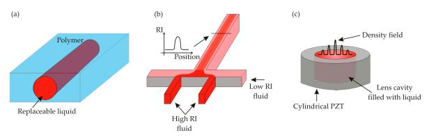
**Figure 3.** (a) A liquid core waveguide which can be tuned by replacing the liquid in the hollow channel; (b) an optofluidic GRIN lens configured by two miscible fluids; and (c) an acoustics-driven gradient refractive index lens.
