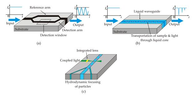
**Figure 6.** Schematics of functional optofluidic devices: (**a**) integrated Mach–Zehnder interferometer for label-free detection of biochemical sample; (**b**) optofluidic enhanced Raman spectroscopy for analytical chemistry; and (**c**) a typical configuration for optical detection or manipulation of micro-particles.
