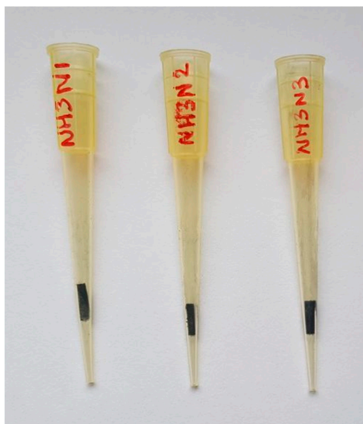
Figure 1. Three different pipette tip extraction units containing carbon nanohorn suprastructures coated over conventional paper as a sorptive phase. The phase is mechanically fixed to the narrower section of the tip and in close contact with its inner walls.
