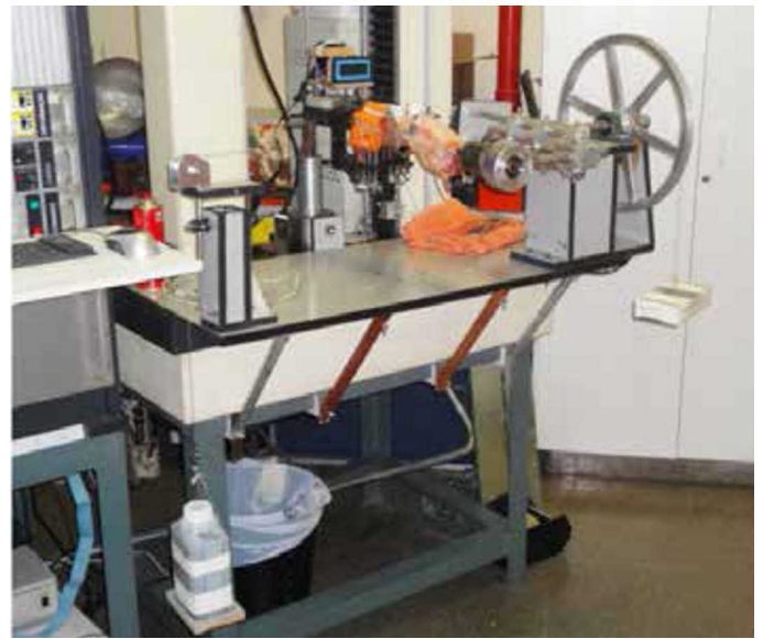
Figure 3 – Right knee fixed to the mechanical device, showing the weight coupled to the pulley (right) and the weight used to lateralize the patella (left).
