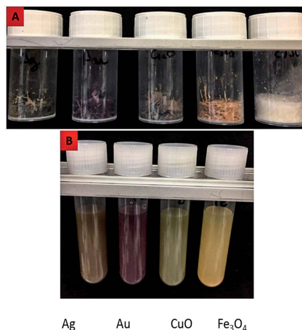
Fig. 4 (A) Dry o/w emulsion of eicosane stabilized with different nanoparticles – from left to right – AgNPs, AuNPs, CuO-NPs, Fe 3 O 4 -NPs, and CNC; (B) o/w emulsion of eicosane stabilized with different nanoparticles (from left to right – AgNPs, AuNPs, CuO-NPs, and Fe 3 O 4 -NPs) after re-dispersion in distilled water (0.05 g mL -1 ).
