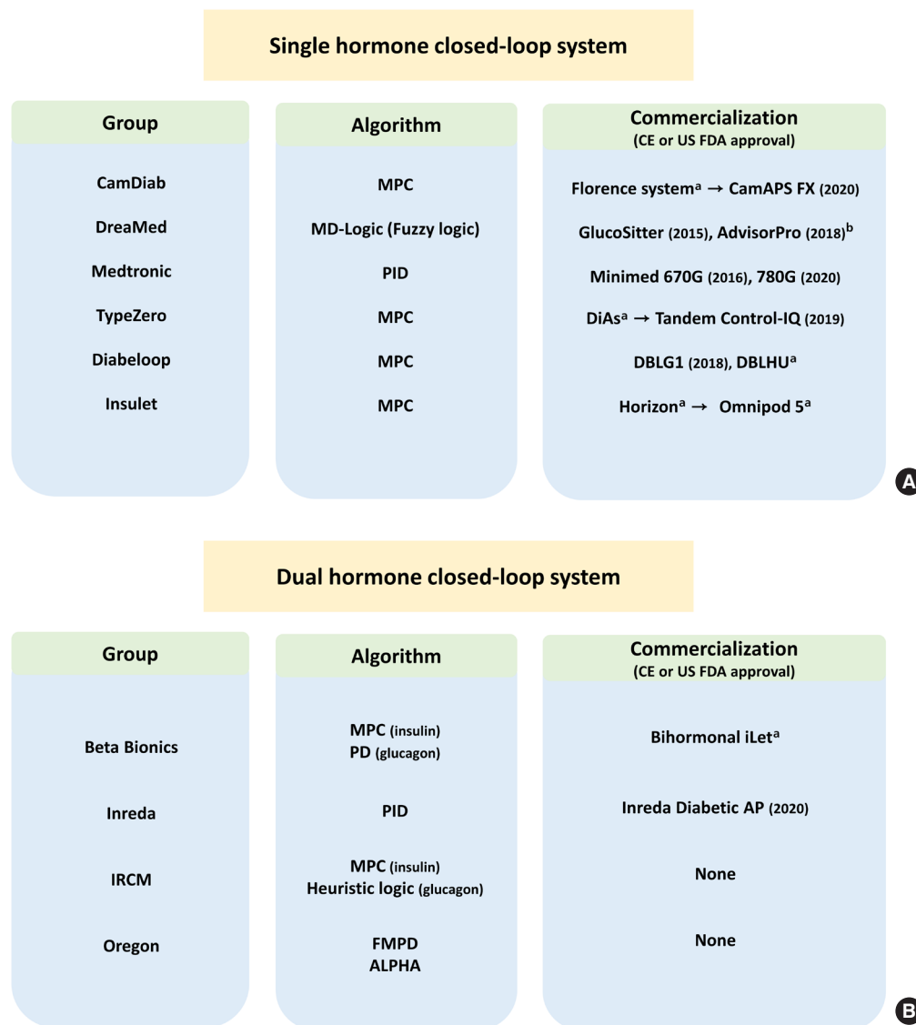
Fig. 4. Schematic diagram of major research groups working on artificial pancreas system. (A) Single-hormone closed-loop system research groups, (B) dual-hormone closed-loop system research groups. MPC, model predictive control; PID, proportional integral derivative control; CE, Conformité Européenne; US FDA, U.S. Food and Drug Administration; DBLG1, Diabeloop Generation 1; DBLHU, Diabeloop for highly unstable diabetes; IRCM, Institut de Recherches Cliniques de Montreal; PD, proportional derivative control; IRCM, Institut de Recherches Cliniques de Montreal; ALPHA, adaptive learning postprandial hypoglycemia prevention algorithm; AP, artificial pancreas. a Not approved yet, b Insulin dosing support system (not closed loop system).
