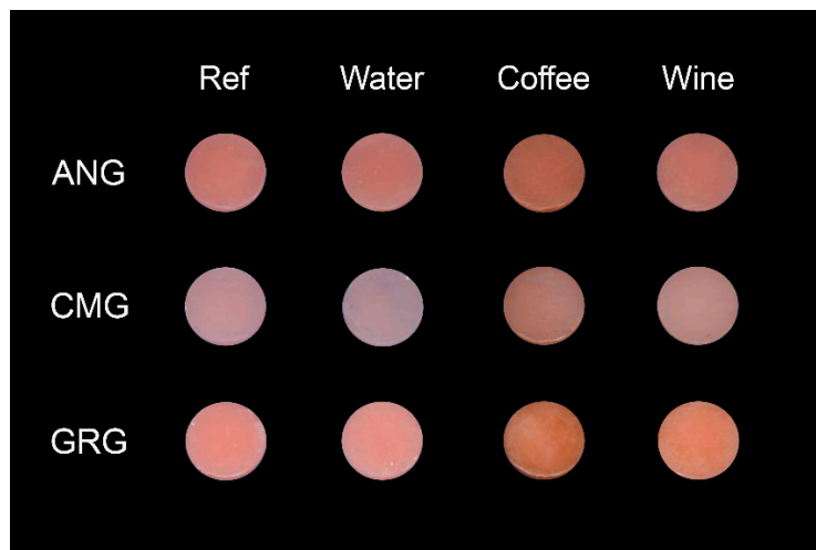
Figure 6. Photograph of the specimens before (ref) and after 30 days immersion in water, coffee and red wine.
