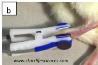
Figure 5 Images displaying the clip sensors used by the pulse oximeter systems. (a) In the base of the mouse or (b) in the centre of the foot in rat. The MouseOx ® murine pulse oximeter system from Starr Life Sciences ® Corp. (Oakmont, PA, USA) provides measurements of O 2 saturation, pulse rate, respiration and pulse and breathe distension. (c) Profile of arterial O 2 saturation measurement in rat during MRI acquisitions at 100% and 21% O 2 during inhalation anaesthesia with isoflurane.
