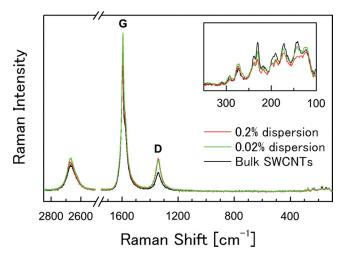
Figure 4. The resonance Raman scattering spectra of bulk SWCNT samples, and 0.2 and 2 mg/mL of SWCNT dispersions in the frequency regions of 100–3000 cm<sup>-1</sup>. The inset shows the spectra of the low frequency region. Abbreviations G and D denote G-band and D-band, respectively.
