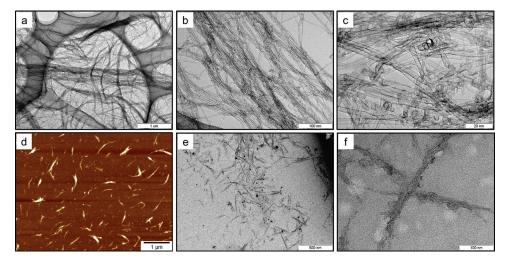
Figure 2. Morphology of the bulk SWCNTs and SWCNTs dispersed in the testing solution. Panels a-c show transmission electron microscopy (TEM) images of bulk SWCNTs at different magnifications. Panel d shows an atomic electron microscopy (AFM) image of SWCNTs dispersed in the testing solution. Panels e and f show TEM images of SWCNTs dispersed in the solution at different magnifications.
