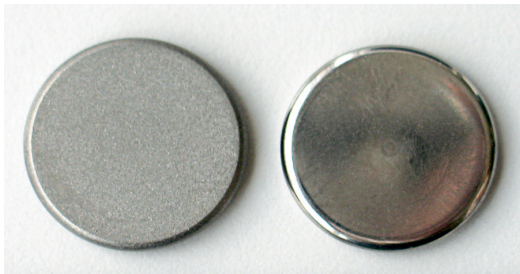
Figure 1. Titanium discs (left) and steel alloy discs (both from Scandinavian Customized Prosthesis AS, Trondheim, Norway) served as surfaces for biofilm formation, with roughness of Ra = 2.5 µm and Ra < 0.5 µm for titanium and steel discs, respectively. All discs were manufactured with a diameter of 17 mm and a thickness of 2 mm.
