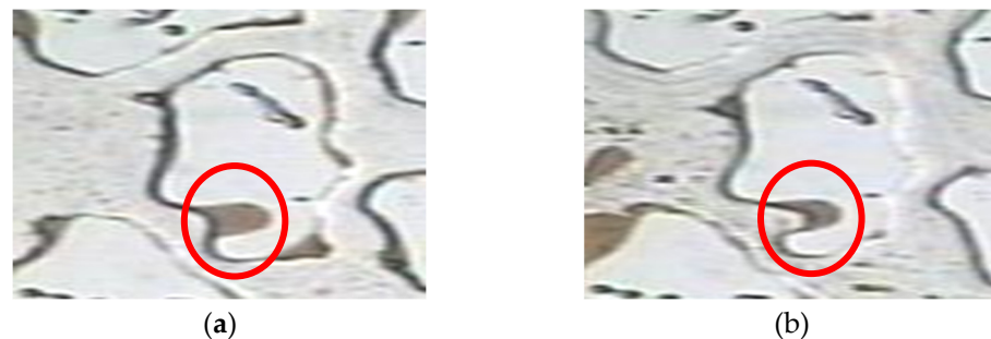
Figure 3. Microscopic images of corner residual oil. (a) After water flooding. (b) After polymer flooding. The corner shaped residual oil is marked in the red circle.
