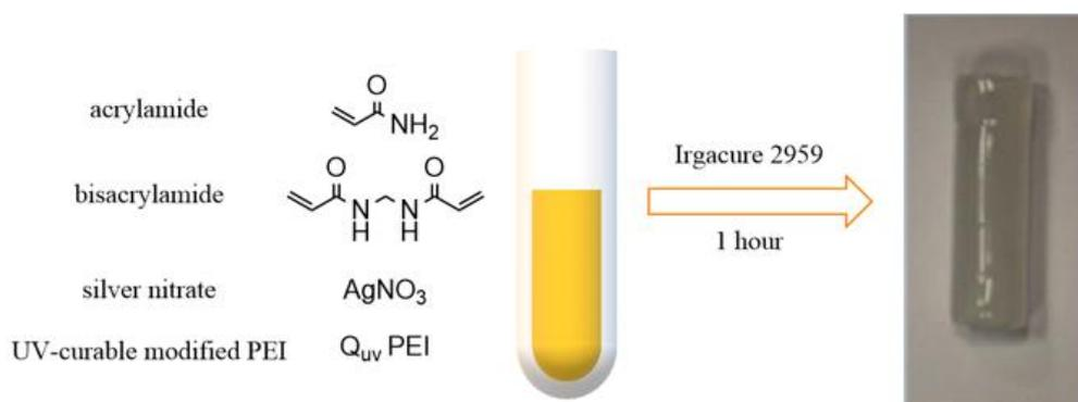
**Figure 12.** Schematic representation of the photoinduced formation of UV-curable cationic poly(ethyleneimine) (Quv-PEI)-based silver-loaded hydrogel. Reprinted with permission. Copyright 2016, Elsevier [44].
