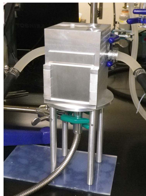
Figure 1 | Custom-made photoelectrochemical cell. Schematic illustration (left) and a photograph (right) are shown. The coolant was set to 20 °C to maintain a constant sample temperature during measurement. d indicates the thickness of the solution layer.
