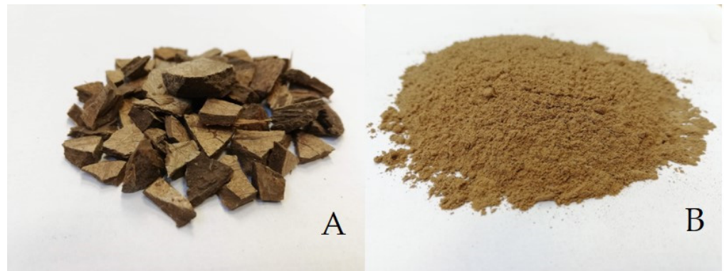
Figure 1. Waste from coconut oil production: (A): pre-crushed coconut shells, (B): natural particulate filler from coconut shells.
