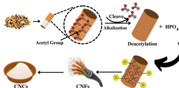
Fig. 1. A diagrammatical illustration of the process of creating Cellulose Nano Crystals (CNC) from cigarette butts. The cigarette filters undergo deacetylation, transforming into Cellulose Nano Fibers (CNFs), which are then processed to produce CNCs.
