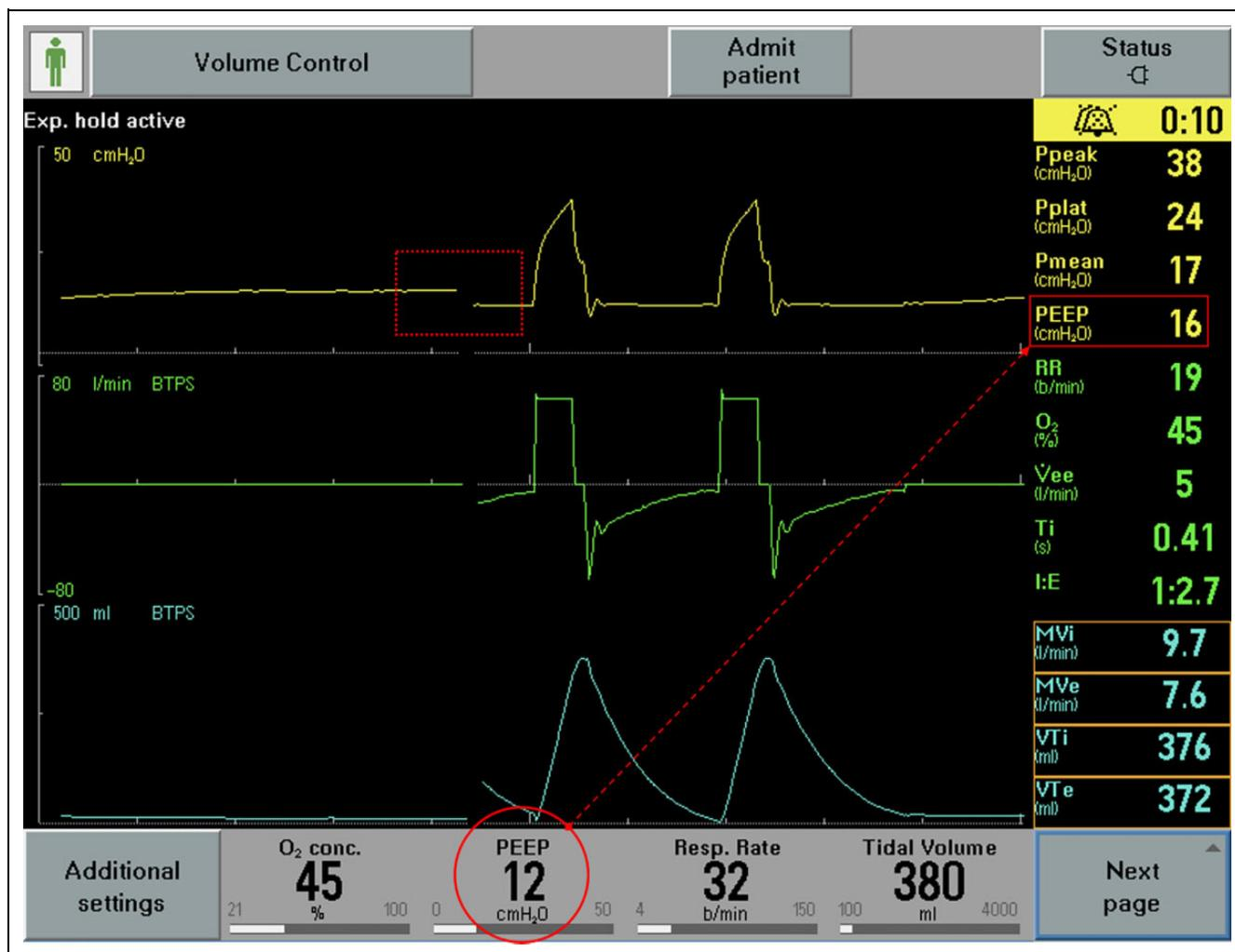
**Figure 3.** Representative image of ventilator waveforms. Intrinsic PEEP unmasked by manual expiratory hold maneuver (dotted rectangle; circle at bottom of the pane represents operator set PEEP and rectangle on the right-hand side of the pane represents PEEP<sub>tot</sub>).
