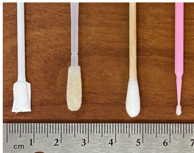
FIGURE 1 Swab types assessed for microbial DNA recovery. From left to right: Luna Innovations Incorporated™ dissolvable swabs (unshaven), Copan FLOQSwabs™, Puritan™ 6" Standard Cotton Swab w/Wooden Handle, and Plasdent™ Maxapplicator™ 'Regular Size' (2.0 mm) Dental Applicators.
