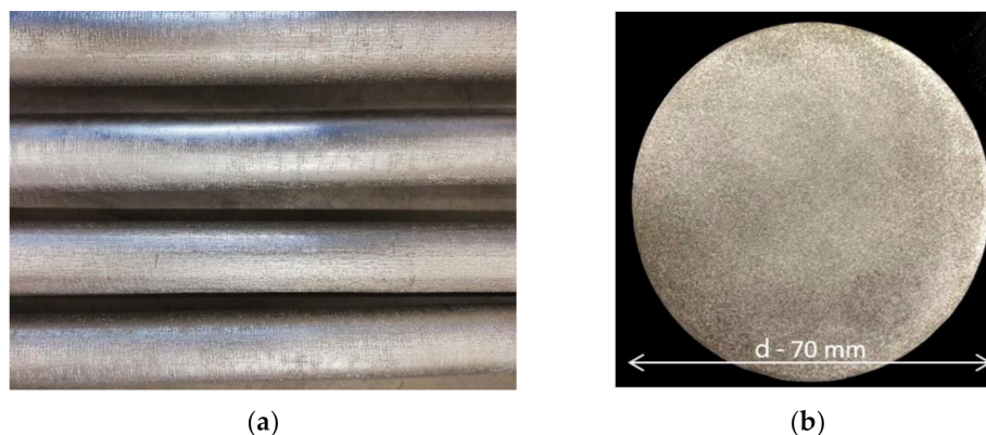
Figure 5. Outer surface of the obtained ingots (a) and a typical macrostructure on the ingot cross section (b).
