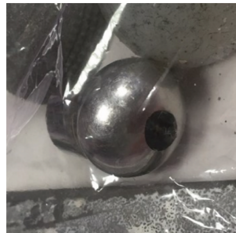
FIGURE 4: Per-operative aspect of the femoral chromium-cobalt head, flattened with a hole in it. 18 g of metal loss explaining metallosis with systemic repercussions.
