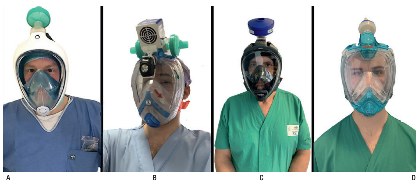
Figure 3. Surgeons wearing four different types of modified snorkelling masks; (A) modified Decathlon mask; (B) Siropack C-Voice mask; (C) Ocean Reef Aria QR+ mask; (D) Seac Unica mask.
