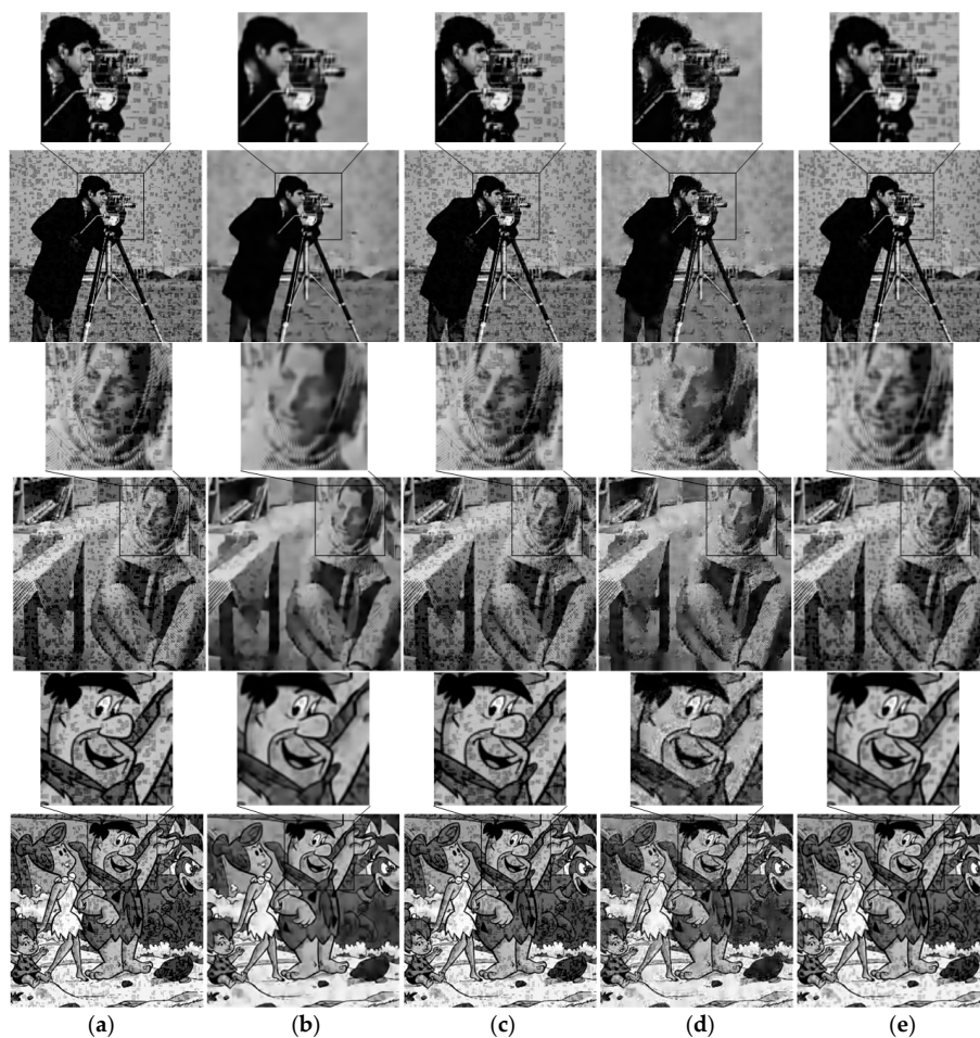
Figure 6. The subjective performance of the proposed structure-preserved sparse coding method: (a) the dataset with simulated clustered noise; (b) the results of proposed method; (c) the results of the method based on DCT; (d) the result of the method based on K-SVD; (e) the result of the method based on BP.
