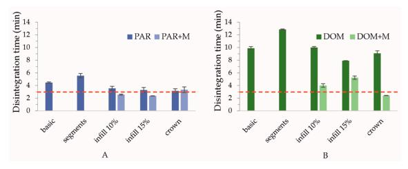
**Figure 3.** Disintegration time of paracetamol- (**A**) and domperidone-loaded tablets (**B**) stored for 24 h in a desiccator ( $22.7 \,^{\circ}$ C, 35% RH). The red dashed line represents the maximum disintegration time of the ODTs according to Ph. Eur.
