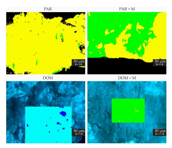
**Figure 9.** Raman maps of tablets made of filaments with different compositions with  $50 \times$  magnification and 4  $\mu$ m step used. Yellow is for APIs in amorphous form, green for crystalline, blue for crospovidone, cyan for PVA, and black for wax or unidentified spectra.
