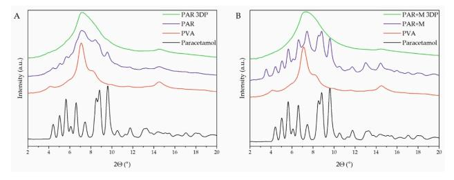
**Figure 6.** XRPD diffractograms of raw paracetamol, PAR (**A**) and PAR + M (**B**) filaments, and 3D printed tablets made of PAR (**A**) and PAR + M (**B**) filaments.
