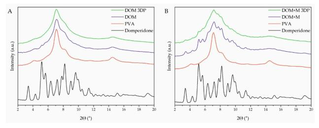
**Figure 7.** XRPD diffractograms of raw domperidone, DOM (**A**) and DOM + M (**B**) filaments, and 3D printed tablets made of DOM (**A**) and DOM + M (**B**) filaments.
