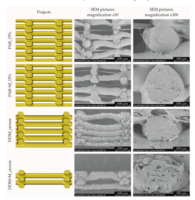
**Figure 4.** Tablets cross-sections based on designs received by reversed voxelization and SEM pictures (magnification  $50 \times$  and  $300 \times$ ).
