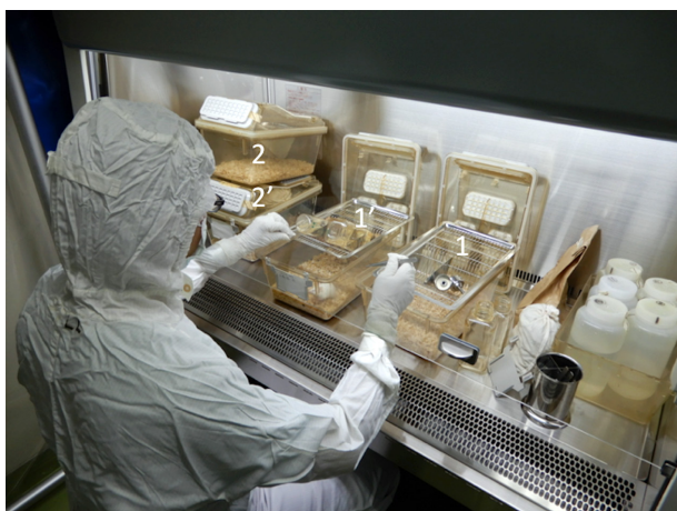
Fig. 8. Cage-change procedure in the safety cabinet. The safety cabinet contained two in-use (1', 2') and two replacement cages (1, 2). Mouse transfer followed the procedure in Fig. 6b. This method was used in Evaluation 3.
