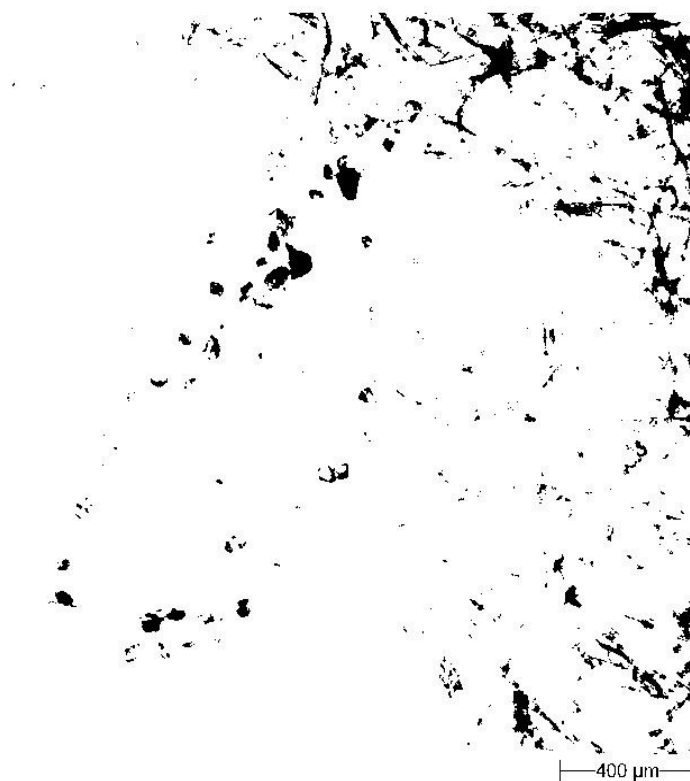
Figure 3. The same soil particles as Figure 2 after filtration of the blotting paper texture at the 0.32 grey level.
