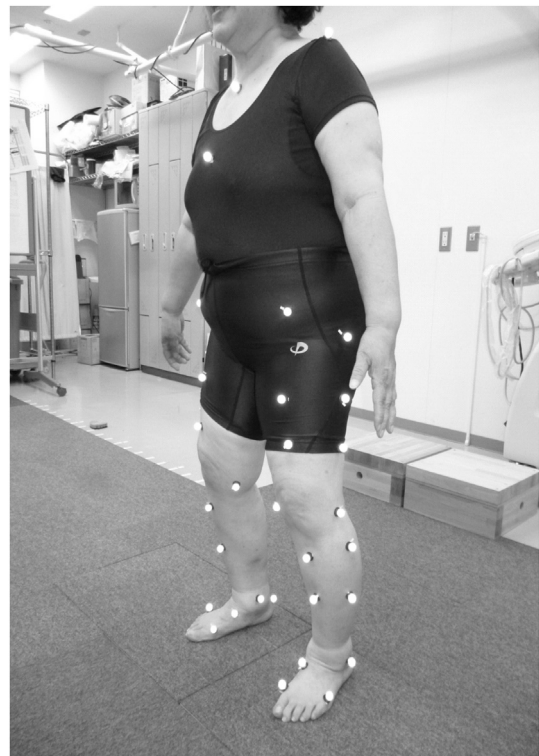
Fig. 1. A total of 46 retro-reflective markers were placed at the standard anatomical landmarks.
