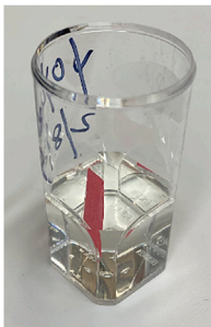
YOYO-1 staining: a coverslip combed with DNA is dropped into YOYO-1 solution.
