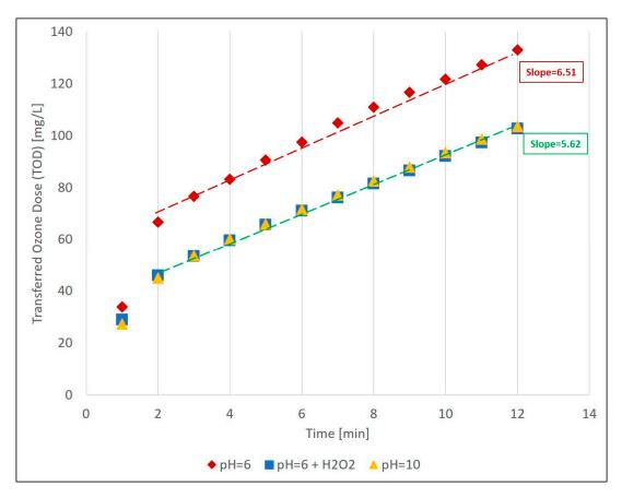
**Figure 4.** Dynamic progress of ozone consumption (as transferred ozone dose (TOD)) for the three studied conditions at 12 min interval. Slopes are calculated beween 2–12 min.
