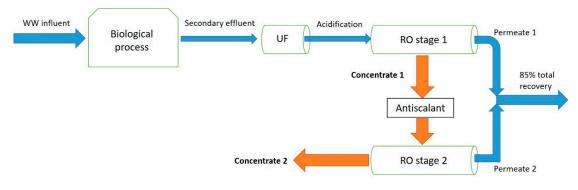
**Figure 1.** Schematic diagram of Bioreactor– ultrafiltration (UF)–reverse osmosis (RO)–RO Nir-Etzion wastewater treatment plant (WWTP) pilot system.
