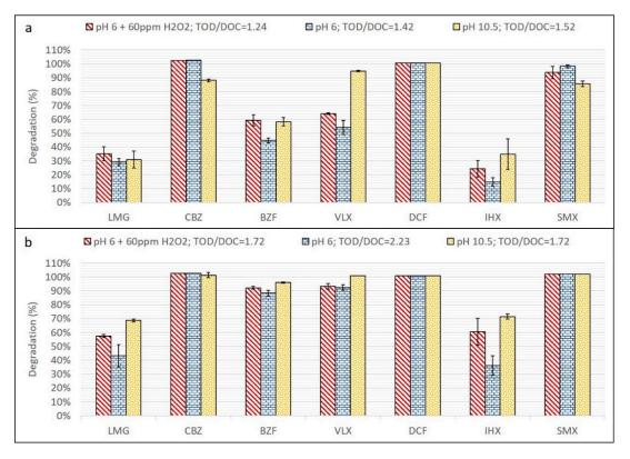
**Figure 3.** Results of degradation by ozone for comparative experiments: (**a**) 5 min ozonation and (**b**) 12 min ozonation.
