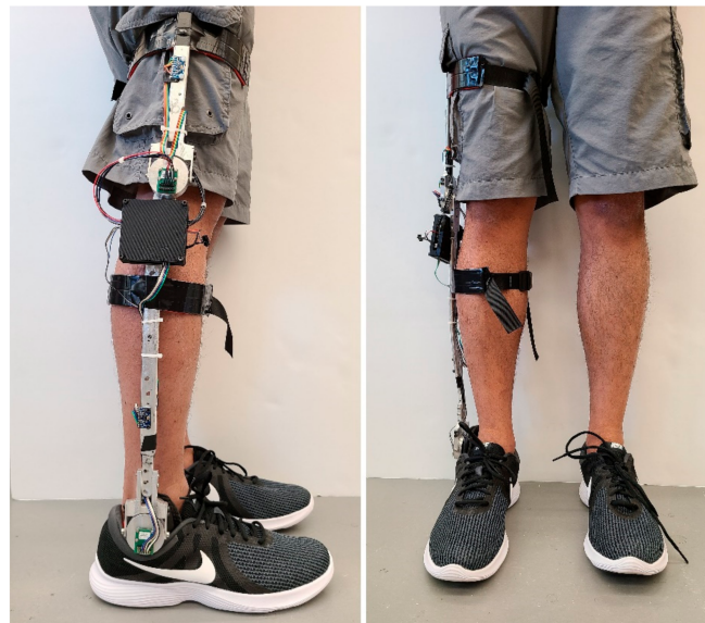
Figure 4. Prototype of the measurement exo-skeleton.
