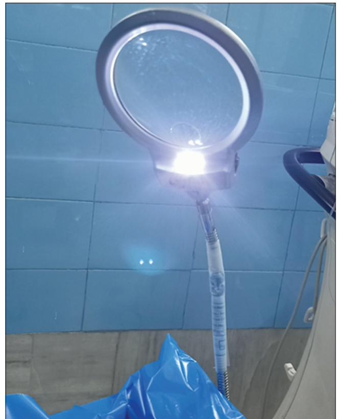
Figure 4: Image depicting a magnifier wrapped with a sterile plastic surgical drape attached at one end of the surgical trolley, a light source for illumination, and a small black button at right bottom end for switching on and off the light
