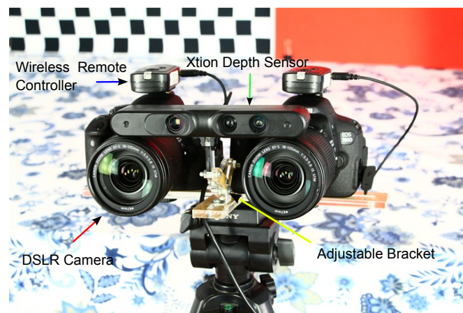
Figure 1. The system used in our method. It consists of two Canon EOS 700D digital single-lens reflex (DSLR) cameras and one Xtion depth sensor. All DSLR cameras are controlled by the wireless remote controller. We used an adjustable bracket to change the angle and height of the Xtion depth sensor.
