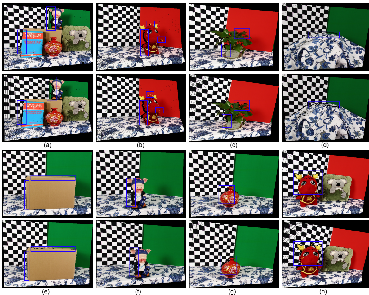
Figure 9. Comparative results for 3D reconstructions. (a) Book; (b) Dragon; (c) Plant; (d) Tablecloth; (e) Box; (f) Piggy; (g) Vase; (h) Dragon and Kola. Each scene from top to bottom contains the reconstruction using our method and the result using the up-sampled disparity map captured by the Xtion depth sensor.
