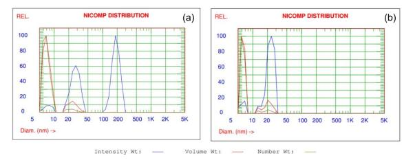
**Figure 3.** Nicomp distribution analysis of the intensity-, volume- and number-weighted data collected for (**a**) ZnO and (**b**) TiO<sub>2</sub> NPs in commercial dispersions.
