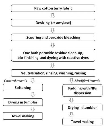
Figure 1. Schematic representation of finishing processes.
