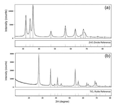
Figure 2. XRD patterns of (a) ZnO and (b) TiO<sub>2</sub> NPs commercial dispersion.
