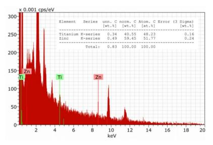
Figure 5. Example of EDX spectra of cotton terry towels modified with ZnO and TiO<sub>2</sub> NPs.
