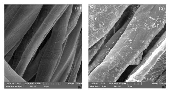
Figure 4. SEM images of (a) unmodified and (b) ZnO and TiO<sub>2</sub> modified cotton terry towels.
