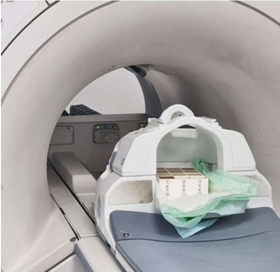
FIGURE 2 The phantom container positioned on the magnetic resonance imaging (MRI) table within the posterior head and face part of the head/neck/spine (HNS) coil
