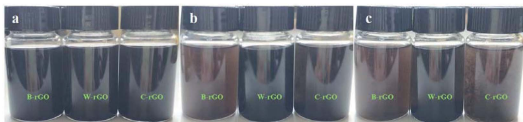
Fig. 8 Static diagram of three rGO nanofluids with a water/ethanol-based solution (25 : 75): (a) 10 days, (b) 20 days, (c) 30 days.
