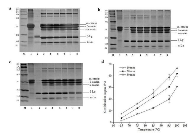
**Fig. 3. SDS-PAGE and combination degree of whey protein and casein in different temperature of heat-treated milk.** a, b and c SDS-PAGE of whey proteins of heat-treated milk for 10 min, 20 min and 30 min respectively. *lane M*: Marker, *lane 1*: casein, *lane 2*: whey protein, *lane 3*: raw milk, *lanes 4 to 8*: 65°C, 75°C, 85°C, 95°C and 100°C. d Combination degree of whey protein and casein (10 min (*white squares*), 20 min (*black circles*), 30 min (*white triangles*)).
