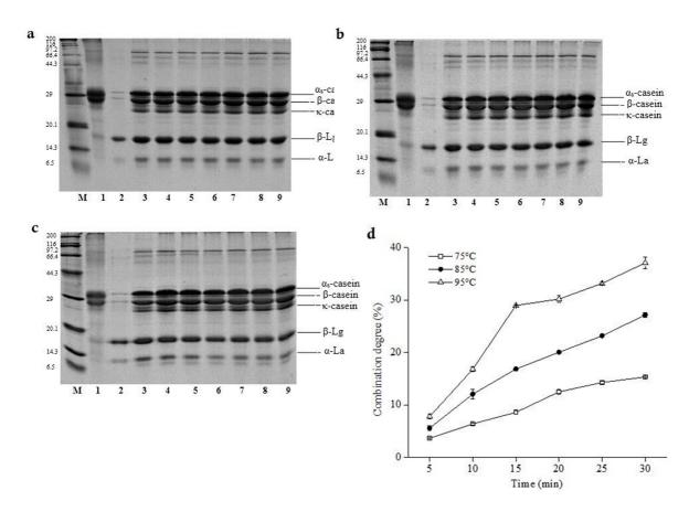
**Fig. 4. SDS-PAGE and combination degree of whey protein and casein in different temperature of heat-treated milk.** a, b and c SDS-PAGE of whey proteins of heat-treated milk for 75°C, 85°C, 95°C respectively. *lane M*: Marker, *lane 1*: casein, *lane 2*: whey protein, *lane 3*: raw milk, *lanes 4 to 9*: 5 min, 10 min, 15 min, 20 min, 25 min, 30 min. d Combination degree of whey protein and casein (75°C (*white squares*), 85°C (*black circles*), 95°C (*white triangles*)).
