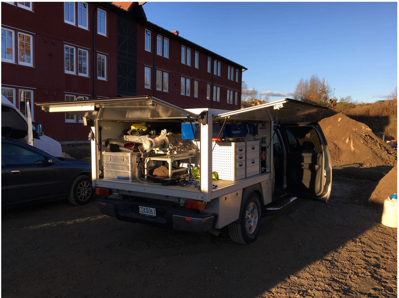
Fig 1. A picture of service-bed compartment of the gamma spectrometry vehicle used in the experiment. The 123% relative efficiency HPGe detector with its nitrogen dewar is visible in the centre-back of the service-bed. The two blue boxes in the upper-right part of the service-bed are the two 4l NaI(Tl) detectors. The GNSS receiver was mounted on the roof of the cabin, above the front passenger.
