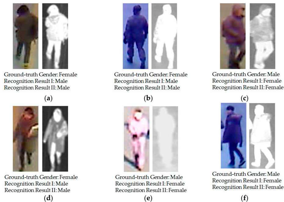
Figure 10. Example of recognition results of our proposed method where the error cases were occurred: (a,b) female images in back view; (c,f) male images in side view; (d) female image in front view; and (e) male image in front view.
