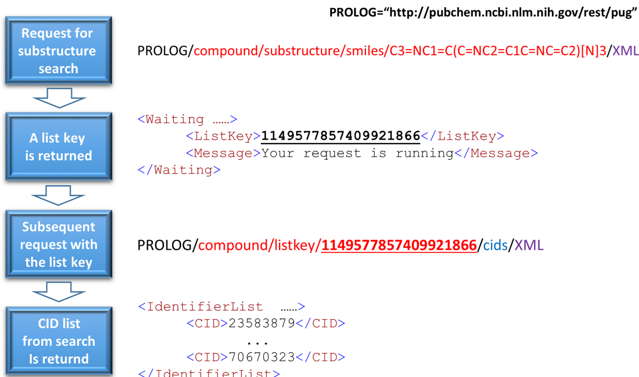
Figure 3. Asynchronous substructure search using the PUG-REST interface. The list key returned from the initial request will be used both to check the status of the search and to retrieve the final results.
